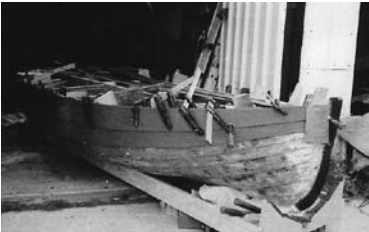
While the boat was upright two new planks were fitted
