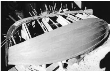
With the boat turned over the rest of the planks were removed and replaced
